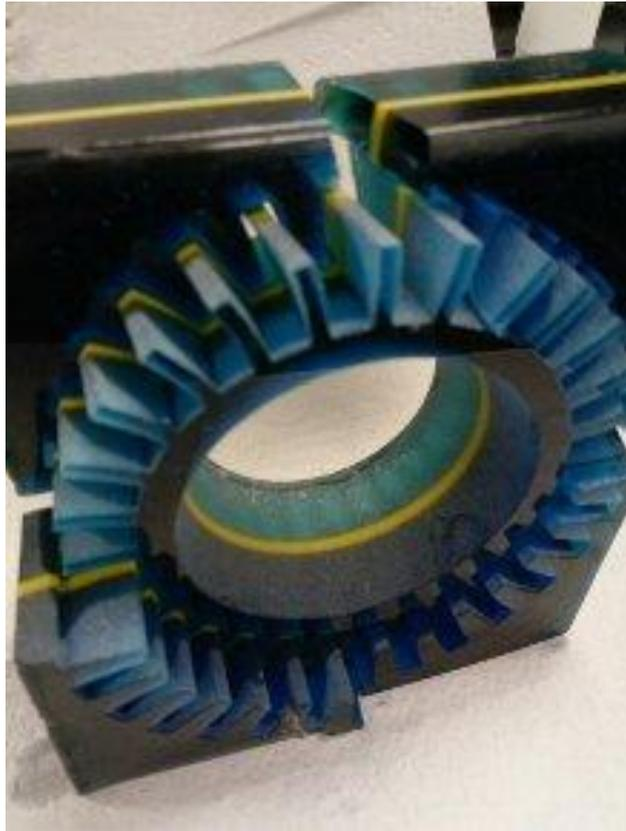
*Experimenting with 5 axis cutting raised issues about how one form can be removed from a block of material - taper lock!*
