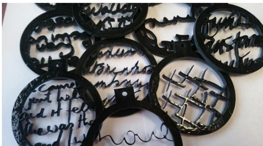
*Details of glass medals prior to being kiln-formed. This demonstrates the complexity of cutting and the ability of the machine to capture the nuances of an individual's handwriting*
